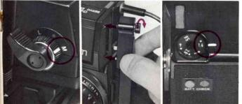
11 When the lens speed adjustment dial is turned, the f/stop scale of the meter reading window slides and the lens speed is indicated just below the under-exposure warning mark as a maximum f/stop.
